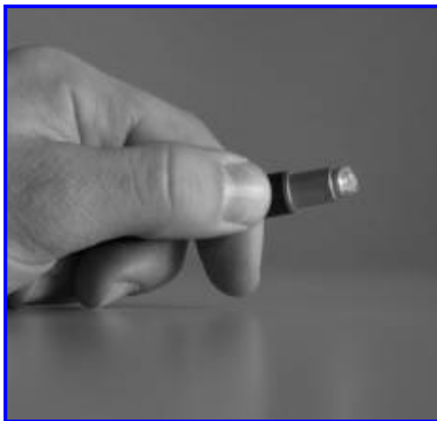
Figure 2. Our modification of a laser pointer. A small piece of transparent green or red plastic is attached to the laser pointer. The modification was invented in order to get better visibility from different viewpoints. However primitive a solution it is, it does the job very well.
